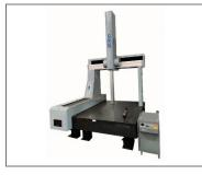
Mitutoyo 9166 CMM with Hexagon control Motorised Indexing Probe TTP Touch Trigger Probing and Scanning with PC-DMIS Measuring Capacity 900 x 1600 x 600
